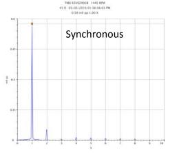
Applying a window (e.g. Hanning) to the data will improve the asynchronous spectrum accuracy to a point, but it will still be significantly less accurate than the synchronous data. Likewise, choosing a lower spectrum resolution will improve the asynchronous spectrum as the buckets will be wider and since the spectrum is calculated over a shorter time interval the speed will have changed less.
