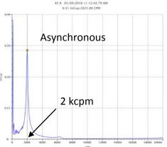
rate still provides good resolution around running speed and the asynchronous spectrum provides information out to higher resonances, blade passage frequencies, etc.
