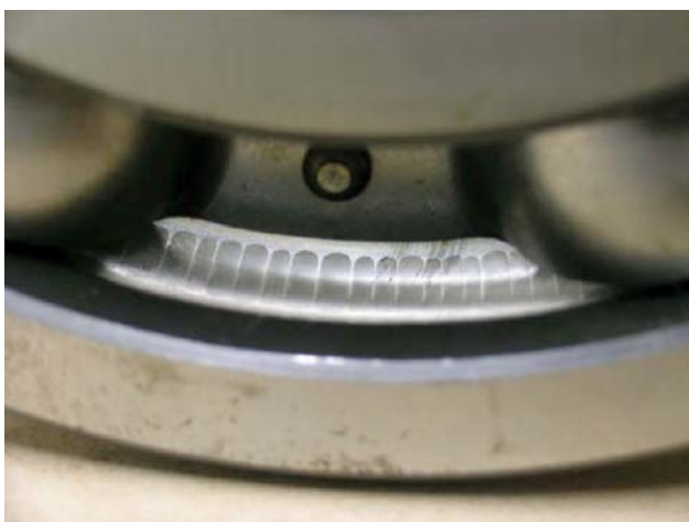
Figure 5: Typical pattern seen on a bearing experiencing fluting
