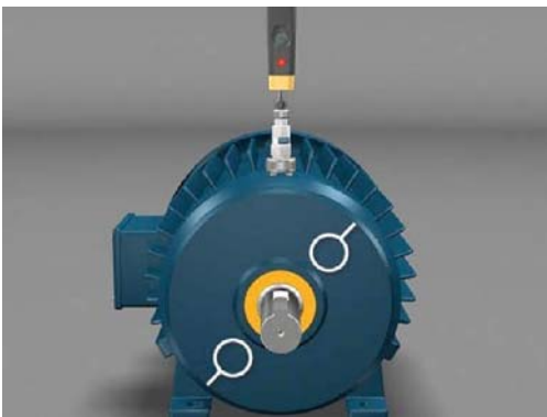
Figure 4: Phase changes when bearing is cocked in the housing
