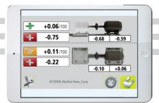
Rotate the sensors to 3:00, measure. The results will be displayed on screen.
