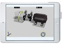
Rotate the sensors to the 12:00 position.Press the measurement icon again to take the second measurement.
