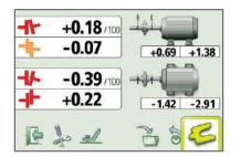
Rotate the sensors to the third position and measure. The results will be displayed on screen. Press the shim icon.
