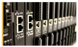
In this issue of VIEWpoint, we're pleased to introduce  $CMS_{SD}$  – the ability for a SETPOINT rack to act as a completely selfcontained flight recorder, streaming highresolution vibration data onto an SD card and holding about one month of data – *including waveforms*. It's unlike anything the industry has seen before because it eliminates the need for *any* condition monitoring software infrastructure at all. No severs, no networks, no IT.
