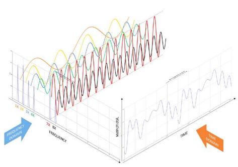
Figure 1: Vibration waveform showing relationship between time and frequency domains.
